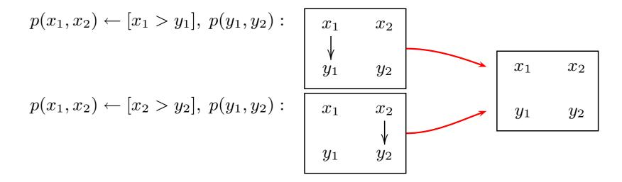
A composition  $\mu_1(\bar{x}, \bar{y}) \circ \mu_2(\bar{x}, \bar{y})$  is a size-change graph entailed by  $\exists \bar{z}.\mu_1(\bar{x}, \bar{z}) \land \mu_2(\bar{z}, \bar{y})$ . Loop descriptions are closed under composition:  $\mu_1 \in G^* \land \mu_2 \in G^* \Rightarrow \mu_1 \circ \mu_2 \in G^*$
